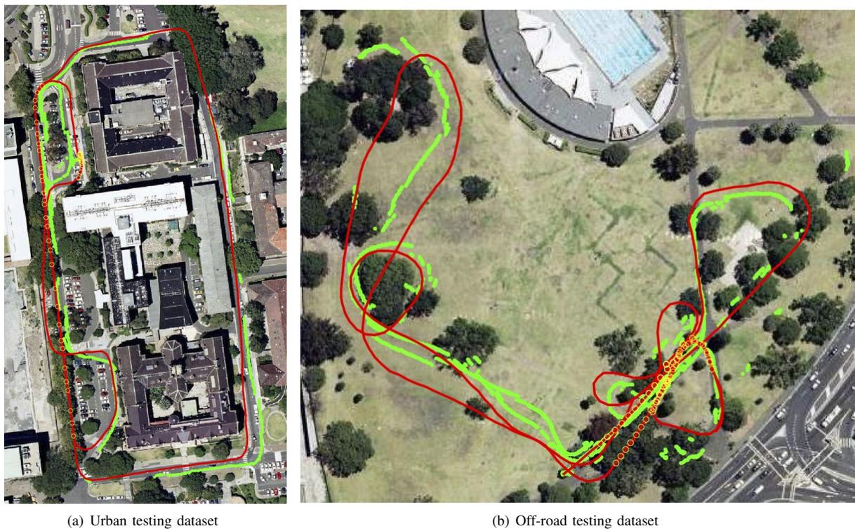
Fig. 6. Localization results obtained using different methods (green dots are GPS information, red lines are visual odometry estimates and yellow circles represent loop-closures).
